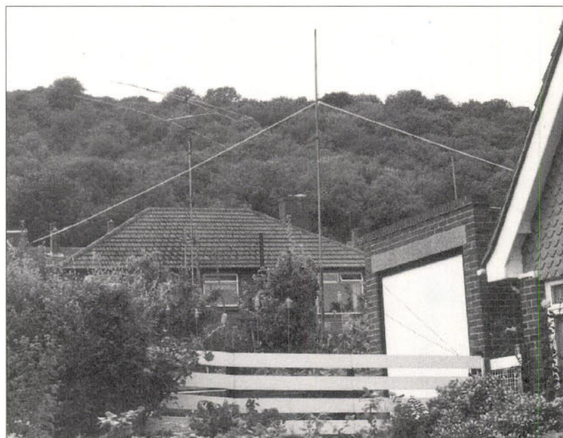
The MyDEL antenna (centre) on test. The low visual impact of the antenna is clearly demonstrated by the photograph itself, when compared to the support mast (see text).
